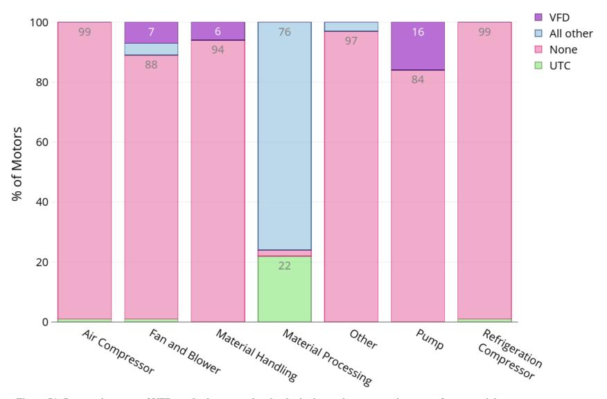
Figure 71: Penetration rates of VFDs and other control technologies by equipment type in terms of commercial motor system counts.
