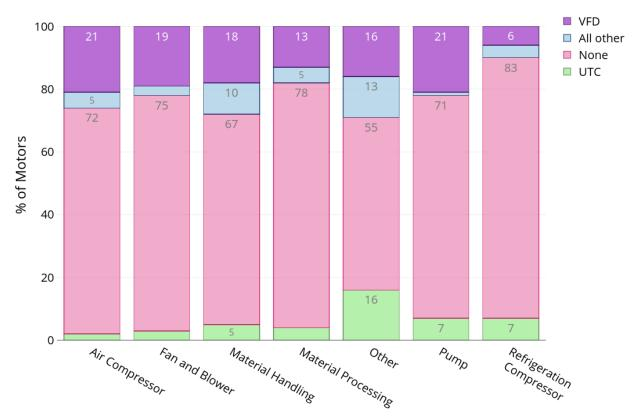
Figure 64: Penetration rates of VFDs and other control technologies by equipment type in terms of industrial motor system counts. Annotations show the corresponding percent for each segment for shares greater than 5%.
