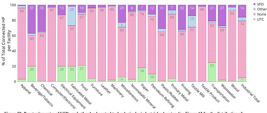
Figure 59: Penetration rates of VFDs and other load control technologies by industrial subsector. See Figure 12 for the distribution of connect hp per facility for the industrial subsectors. Annotations show the corresponding percent for each segment for shares greater than 5%.
