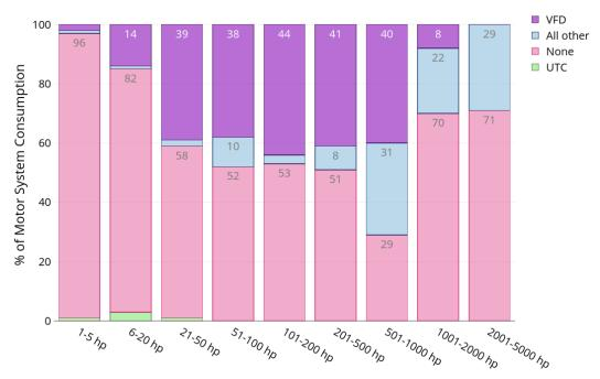
Figure 68: Penetration rates of VFDs and other control technologies by motor size in terms of percentage of commercial sector motor system electricity consumption. Annotations show the corresponding percent for each segment for shares greater than 5%.
