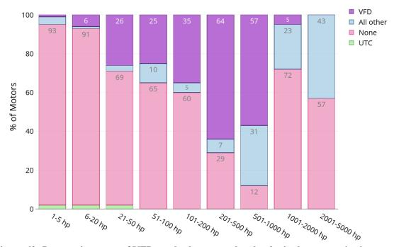
Figure 69: Penetration rates of VFDs and other control technologies by motor size in terms of percentage of commercial motor system count. Annotations show the corresponding percent for each segment for shares greater than 5%.
