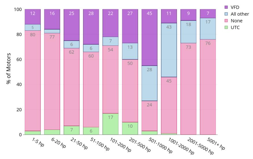
Figure 62: Penetration rates of VFDs and other control technologies by motor size in terms of percentage of industrial motor system counts. See Figure 12 for the distribution of connect hp per facility for the industrial subsectors. Annotations show the corresponding percent for each segment for shares greater than 5%.
