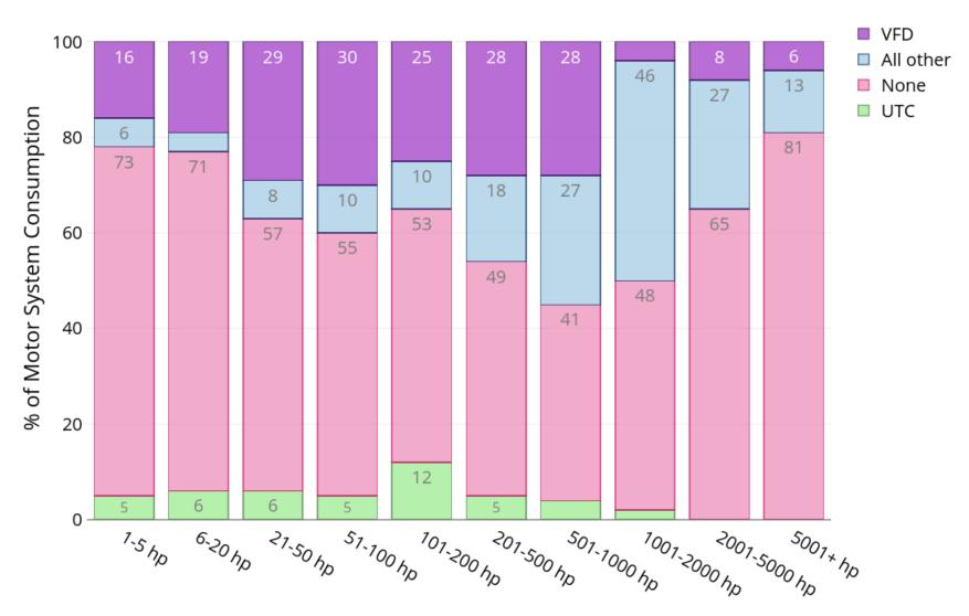
Figure 61: Penetration rates of VFDs and other control technologies by motor size in terms of percentage of industrial motor system electricity consumption. See Figure 12 for the distribution of connect hp per facility for the industrial subsectors. Annotations show the corresponding percent for each segment for shares greater than 5%.
