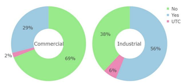
Figure 4: Legibility of nameplates on motors assessed: commercial (L) and industrial (R)
