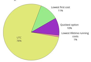
Figure 85: Criteria used for motor repair/replace policy in commercial facilities, percent of facilities
