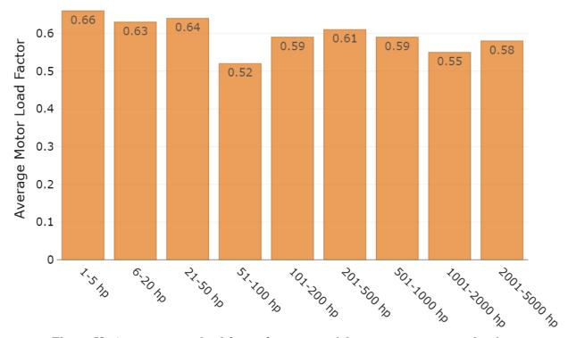
Figure 58: Average motor load factor for commercial sector motor systems by size
