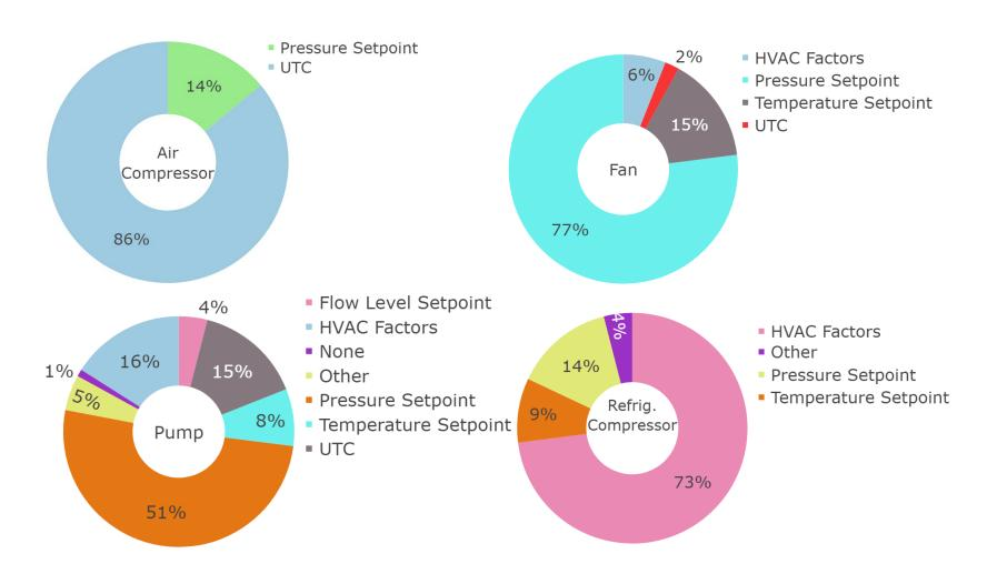
Figure 72: VFD control feedback for commercial air compressors, fans/blowers, pumps, and refrigeration compressor.
