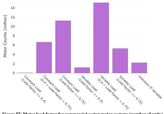
Figure 57: Motor load factor for commercial sector motor systems (number of units)
