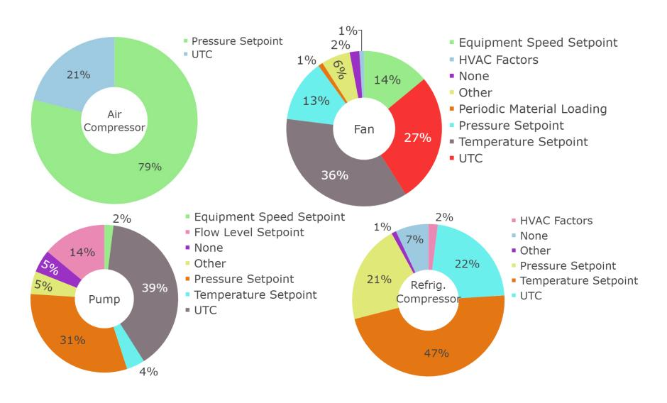
Figure 65: VFD control feedback for industrial air compressors, fans/blowers, pumps, and refrigeration compressors as a percentage of system counts
