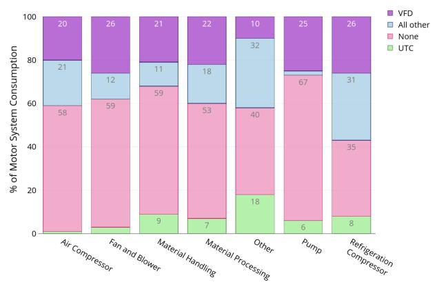
Figure 63: Penetration rates of VFDs and other control technologies by equipment type in terms of industrial motor system electricity consumption. Annotations show the corresponding percent for each segment for shares greater than 5%.
