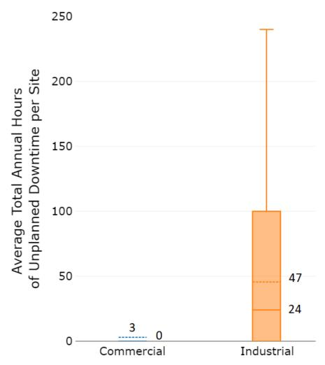
Figure 82: Distribution of annual unplanned system downtime due to motor system failure.
