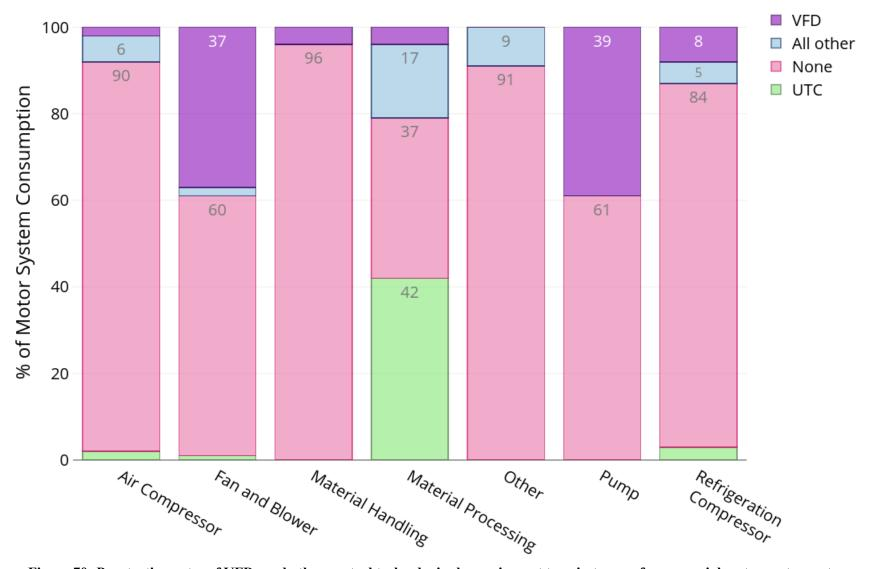
Figure 70: Penetration rates of VFDs and other control technologies by equipment type in terms of commercial sector motor system electricity consumption. Annotations show the corresponding percent for each segment for shares greater than 5%.
